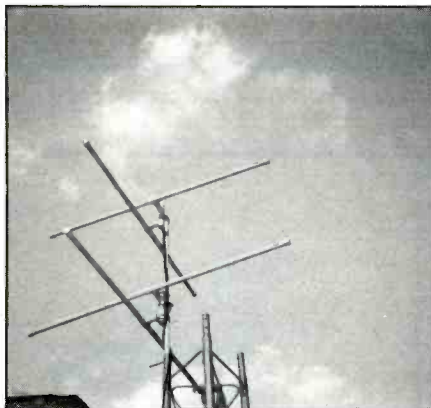
A two element twist for satellite work. Courtesy Ron Burke KB9DJA.
