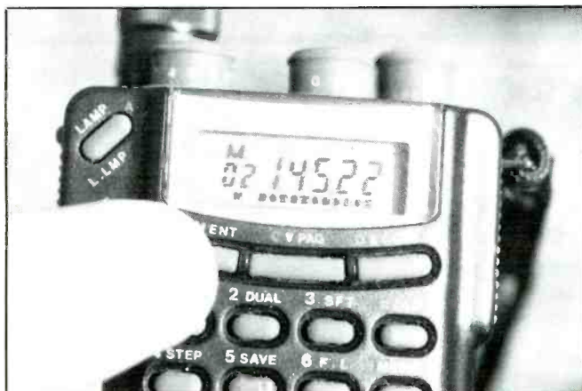
The decode number for personal or group calling is key-pad entered in seconds.
