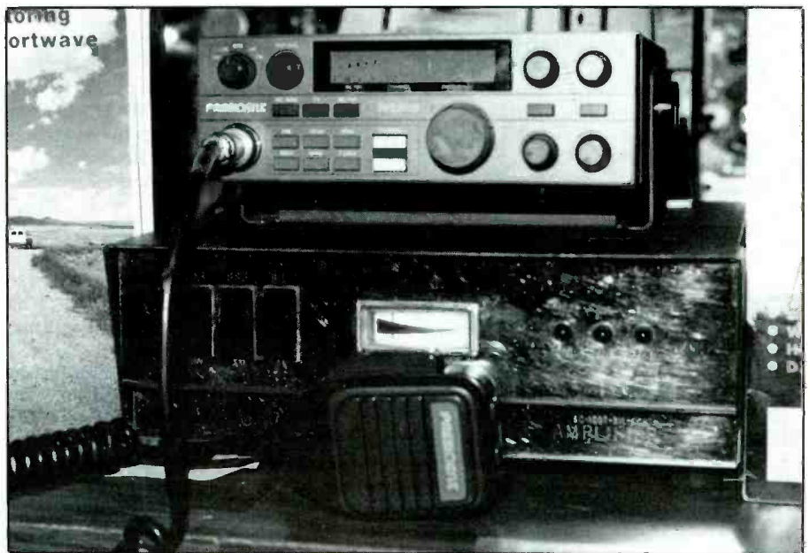
Some 10-Meter ham band SSB transceivers can be modified for unauthorized operation in the 29.80 to 29.995 MHz band, as well as other bootleg frequencies. This modified 25-watt President HR-2510 ham rig is given extra muscle on these channels by the 100 watt linear amplifier it's sitting on.
